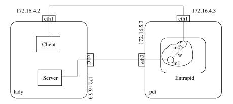
Figure 2: The testbed setting: machine *lady* runs application entities and machine *pdt* runs the *Entrapid*. Routes are set up so that all the traffic between *lady* and *pdt* goes through the virtual link w in *Entrapid*.
