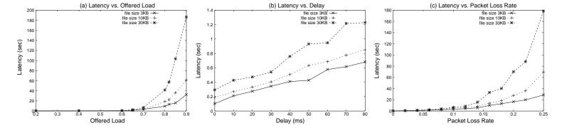
Figure 4: Effect of the network performance on the retrieval latency for different file sizes: (a) Retrieval latency vs. offered load, (b) Retrieval latency vs. packet delay, (c) Retrieval latency vs. packet loss rate.
