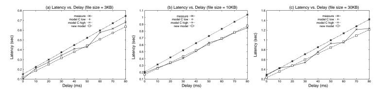
Figure 6: Packet delay vs. retrieval latency (with packet loss rate set to 0): (a) file size = 3KB, (b) file size = 10KB, (c) file size = 30KB.
