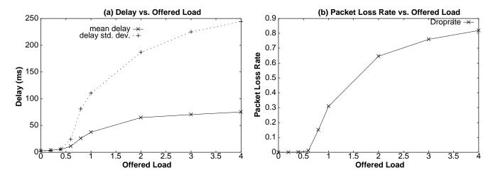
Figure 3: The network performance parameters configuration in our experiments (mean packet size = 512 bytes): (a) mean and variance of packet delay vs. offered load (b) packet loss rate vs. offered load.
