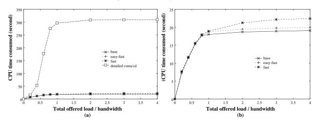
Figure 12: The CPU time consumed for 10 seconds simulations of 10 Mbps Ethernet link with packet size = 512 bytes and buffer size = 8 packets ((b) is the zoomed version of the three curves in the lower portion of (a)).
