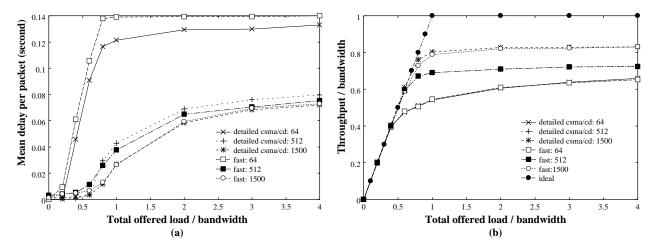
Figure 11: The simulation results for fast Ethernet simulation and CSMA/CD simulation for packet size = 64, 512, and 1500 bytes and buffer size = 4500 bytes: (a) delay versus total offered load, (b) throughput versus total offered load.
