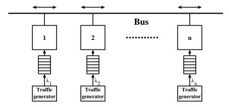
Figure 2: Model configuration for the distributed simulation
