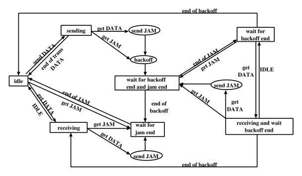
Figure 3: State diagram of distributed CSMA/CD simulation
