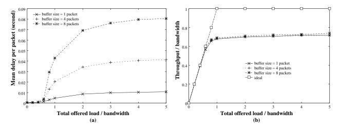
Figure 6: 10 Mbps Ethernet simulation results with buffer size of 1, 4, 8 packets (packet size = 512 bytes): (a) mean delay versus total offered load, (b) throughput versus total offered load.
