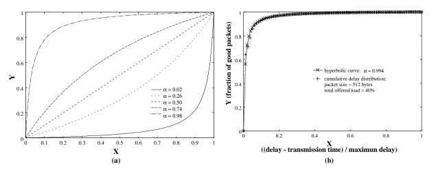
Figure 8: Hyperbolic curves: (a) A group of hyperbolic curves, (b) using hyperbolic curve to model cumulative delay distribution.
