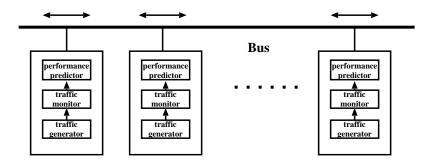
Figure 9: Fast Ethernet simulation configuration.
