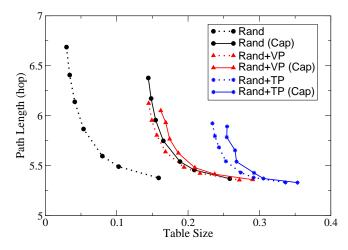
Fig. 7. Tradeoff between average path length and forwarding table size, with the maximum path length capped at 15 hops
