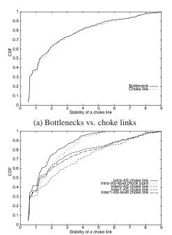
(b) Intra-AS vs. inter-AS choke linksFigure 12: The stability of choke links.
